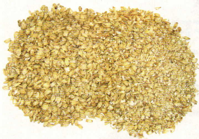
Conditioned (steamed) malt on the left vs. dried malt on the right, after crushing. Note the larger, nearly intact husks in the conditioned malt. These husks, however, are empty.
