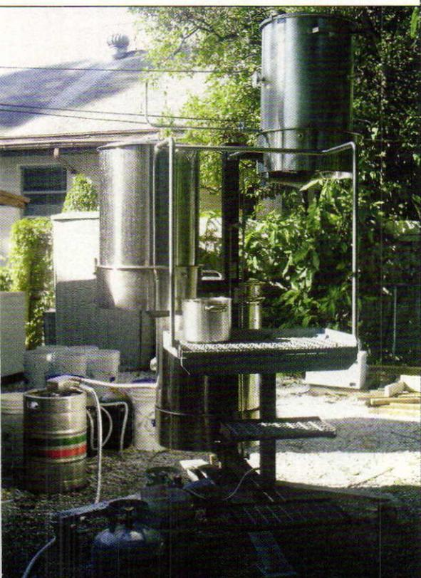
To build the sculpture, the two hit some local scrap yards and found lots of stainless steel. Top to bottom it is about 9 feet (2.7 m) tall, and features steps and landings on the back so that Doug can access the hot liquor tank at the top.
