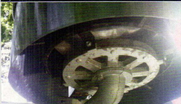
Once Jay figured out the specifications of the tanks, he designed the burners with a flame shroud - which works like a heat shield - so that the tanks could receive enough heat.
