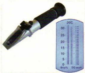
This MoreBeer! refractometer is the first and only model to feature both a Brix Scale and a Specific Gravity Scale so there is no need to convert the reading from Brix (what winemaker's use) to Specific Gravity. Easily used pre-ferment, a refractometer can now easily be used for readings during fermentation with the help of our spreadsheet that includes a video on how to use.
