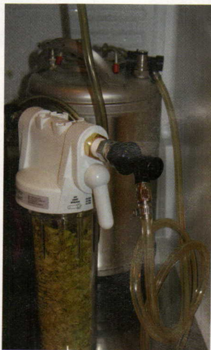
This hop filter project is an easy way to make your keggered homebrew much hoppier.
