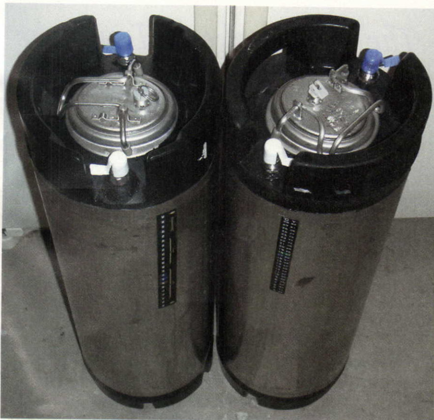
The posts on these kegs, here covered with white and blue caps, are where the gas enters and beer leaves the kegs. You can see the pressure relief valves in the middle of the lids.
