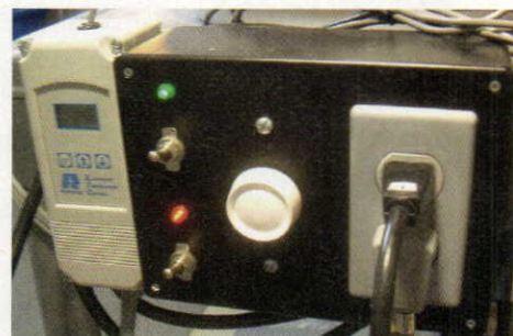
Automated controllers can make decisions in a home brewery that bring about constant mash or fermentation temperatures.
