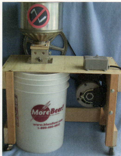
With a few modifications, a Crankandstein grain mill can be converted from hand-crank to motorized.
