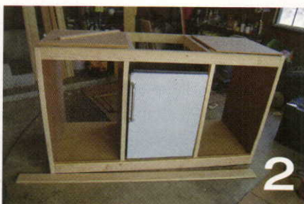
To avoid a surprise later, be sure to test fit the kegerator early in the construction.
