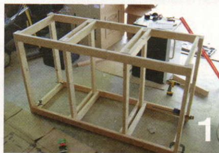
The frame of the bar is constructed from 6-foot, 25-inch and 43½-inch 2x4s.
