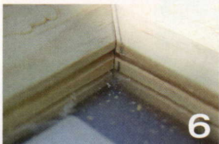
The two slots are spaced far enough apart that one layer of grain will fit between.
