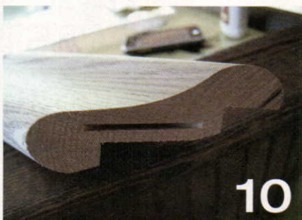
A biscuit joiner was used to join the mouldings used as the armrest on the bar.
