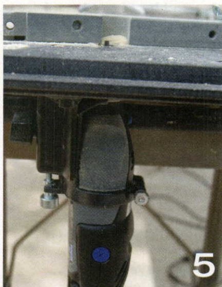
A jig for the Dremel is used to router the grain frame to accept the glass panes.
