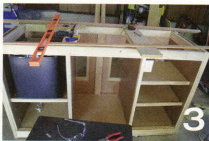
The interior walls and shelves are made of medium density fiberboard (MDF).
