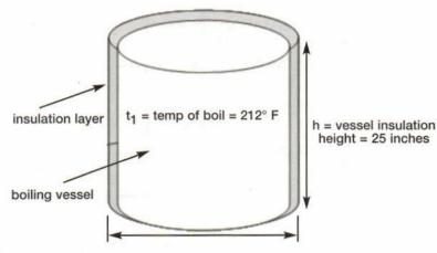
d = diameter of outermost face of insulation = 26 inches (vessel diameter - 22 inches, insulation thickness = 2 inches)
