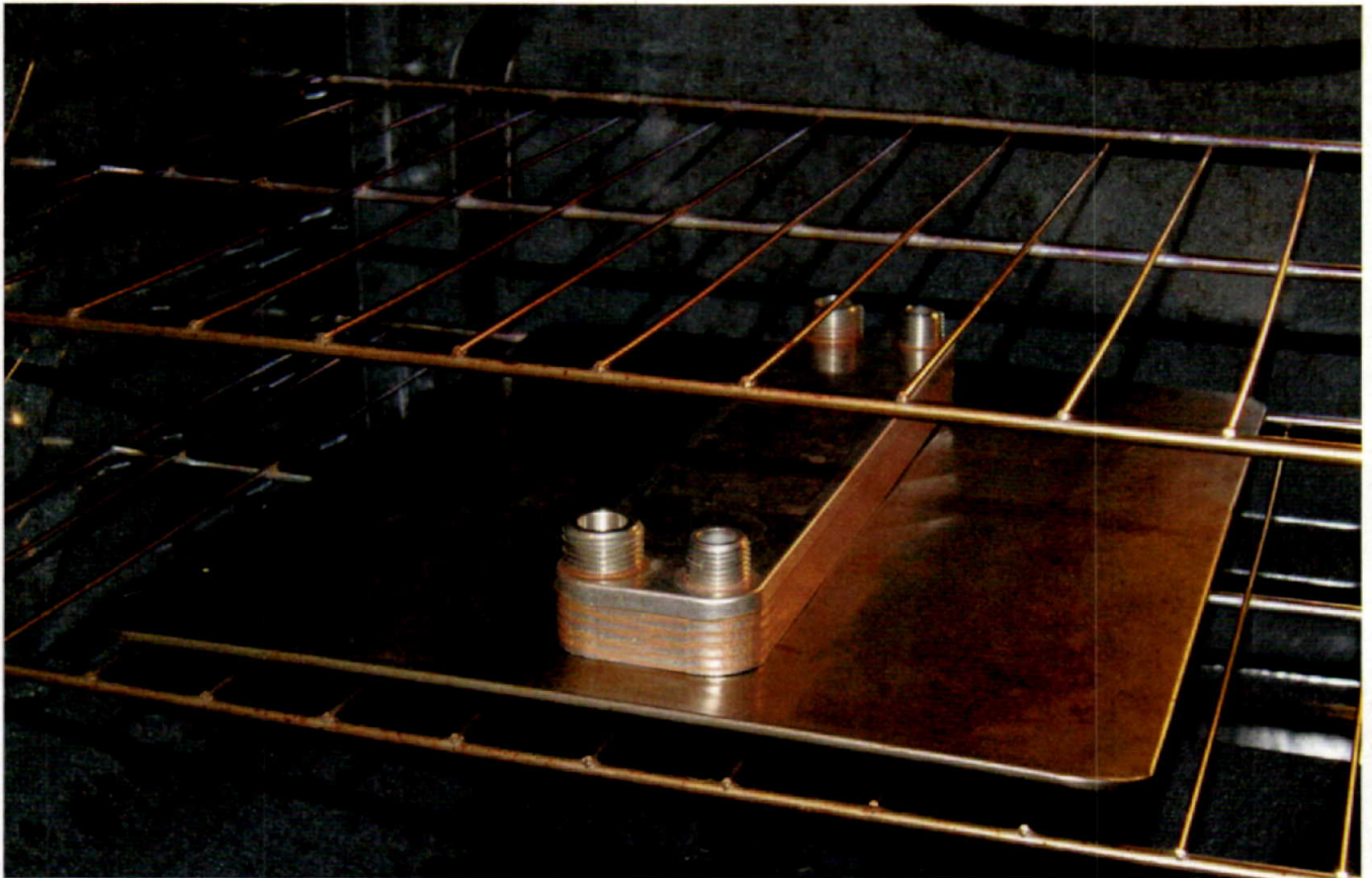
Dry heat can sanitize parts and is a great solution for equipment that has unreachable surfaces (such as this plate chiller). Baking for 60 minutes at 340 °F (170 °C) is required for effective sanitation. Hot liquid can also be used as a sanitizer and contact times are much shorter.
