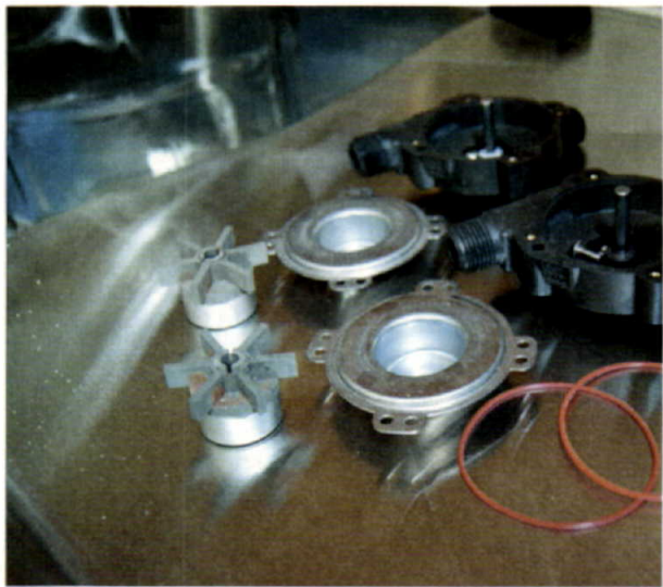
The pump heads for most homebrew pumps are easily disassembled to clean the impeller and inside surfaces.
