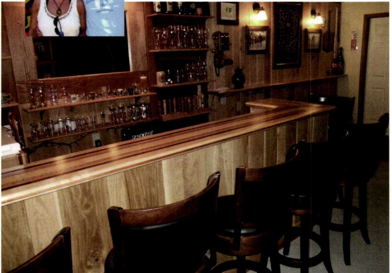
"The bar top is made from maple, mahogany, cherry, white oak and walnut. The bar back is made from 100-year-old doors that I saved from the first house that I owned and the mirror frame is made from wormy oak. I turned the tap handles on my grandfather's 1940s Delta lathe."
