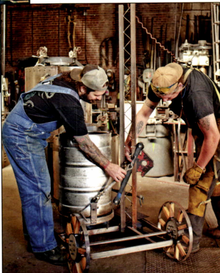
The tower had to be able to hold a full brewing keg — without buckling or tipping, even if bumped — as it was hauled to the top of the brewing rig.
