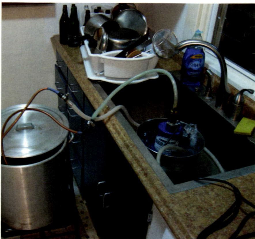
Chilling wort to lager fermentation temperature can be difficult, especially if your tap water is not very cold. Using a pump to recirculate ice water through an immersion chiller is one practical solution to this common problem.
