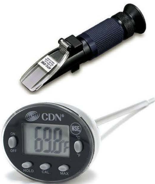
A refractometer (top) and digital thermometer. Both should be calibrated before use.
