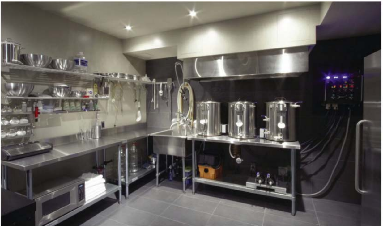
THE BREWERY: "When I designed this new brewing room in 2012, I was able to expand the original brewery to my exact specifications and combine everything relating to brewing (wort creation, fermentation, conditioning, packaging, and serving) into one room, simplifying the brewing process. Commercial stainless steel tables along with an oversized sink equipped with a pre-rinse faucet make for easy cleaning of kegs and kettles."
