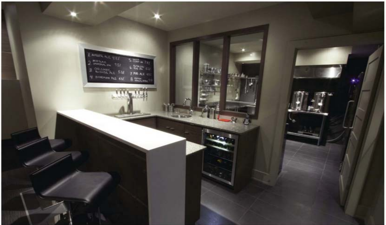
THE BAR: "Eight beers are available on this home tap, served from a keg freezer (keezer) located just inside the brewery. Two of the taps use a nitrogen/CO 2 blend for beer styles that benefit from a creamy Guinness-style pour. The tower and taps are chilled continuously with RV antifreeze that is re-circulated using a pond pump and 50 feet (~50 m) of copper coil located in a separate small freezer."
