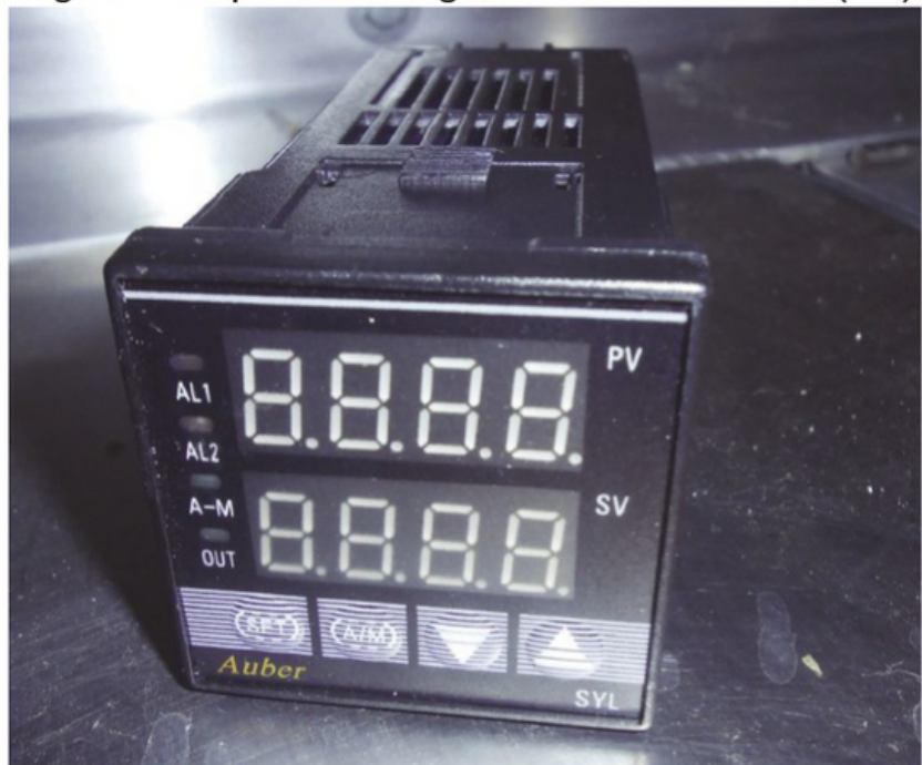
Figure 4: Proportional Integral Derivative controller (PID)
