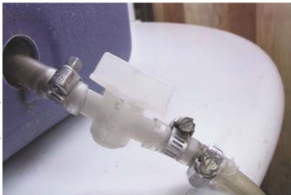
On the outside of the cooler, the braid is attached to a valve that will regulate the flow of wort when you drain the mash tun.
