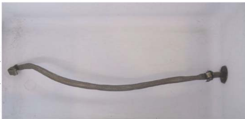
A stainless steel braid made from a water supply line inside of a mash tun will separate the wort from the grains when you drain the cooler. See additional photo on page 54.
