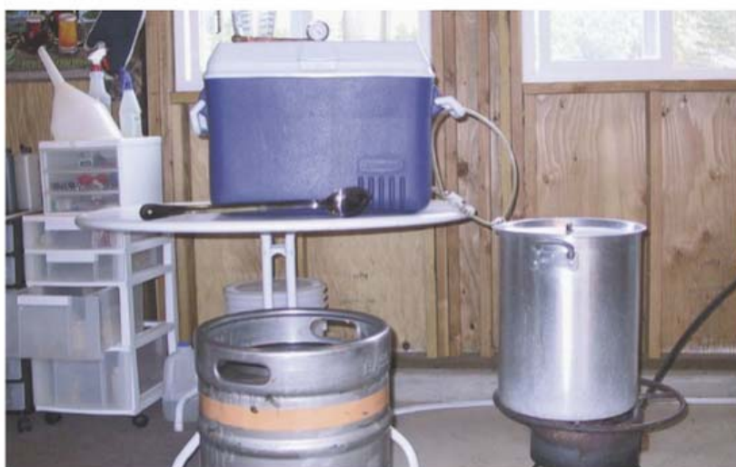
Batch sparging requires very little equipment that most all-grain brewers already have. All you really need is a 5-gallon (19-L) cooler mash tun to brew 5-gallon (19-L) batches.
