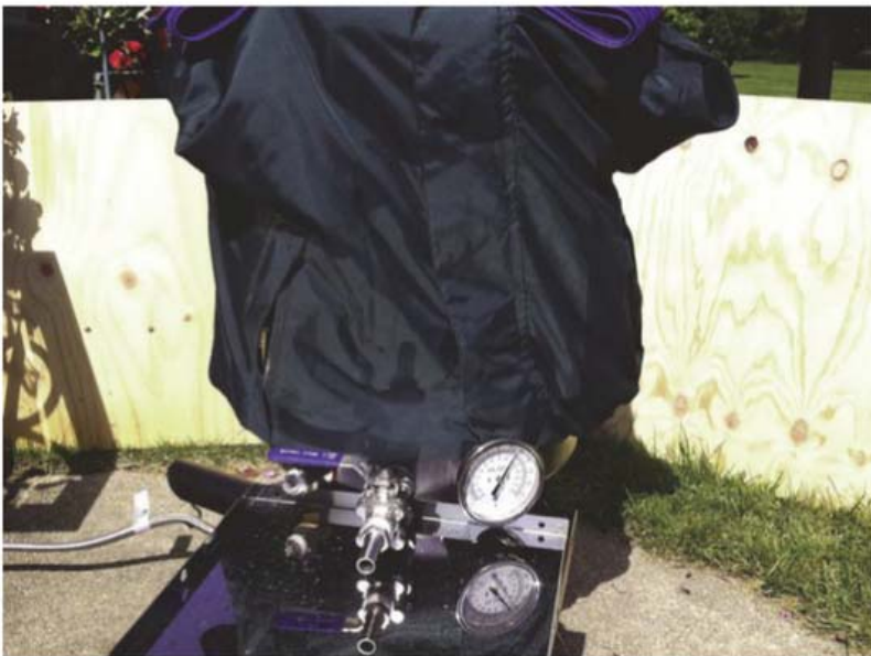
Step 4: Mash the grains for 90 minutes, insulating the kettle to prevent heat loss. A longer mash (as compared to traditional all-grain brewing) can help increase efficiency.
