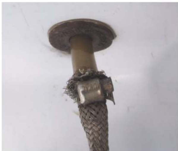
You can attach the stainless steel braid in the mash tun with a bung placed in the drain hole of the cooler.
