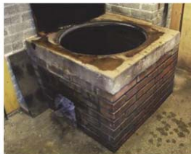
A traditional wood-fire-heated kettle, which is used for making authentic Finnish sahti.
