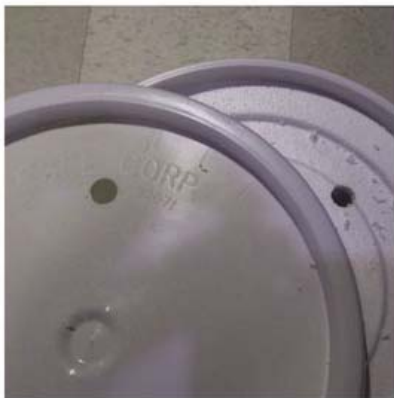
You can easily modify the foam lining and bucket lid to accommodate the beer line.
