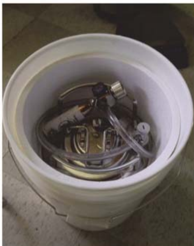
Attach the beer line, regulator and CO 2 supply as you would on a regular setup.
