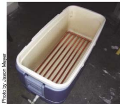
Figure 4. Insulated ice chest used as a mash tun
