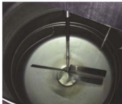
Figure 7. Homebrewing mash mixer with indirect internal heating coil
