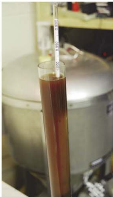
Step Four: Measure the final gravity of the sample, record the results and discard the sample (do not add it back into your main batch of beer).
