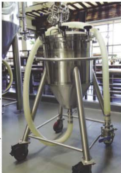
The hop cannon at Pfriem Family Brewers in Hood River, Oregon, which shoots hop pellets into the fermenter using CO 2 .
