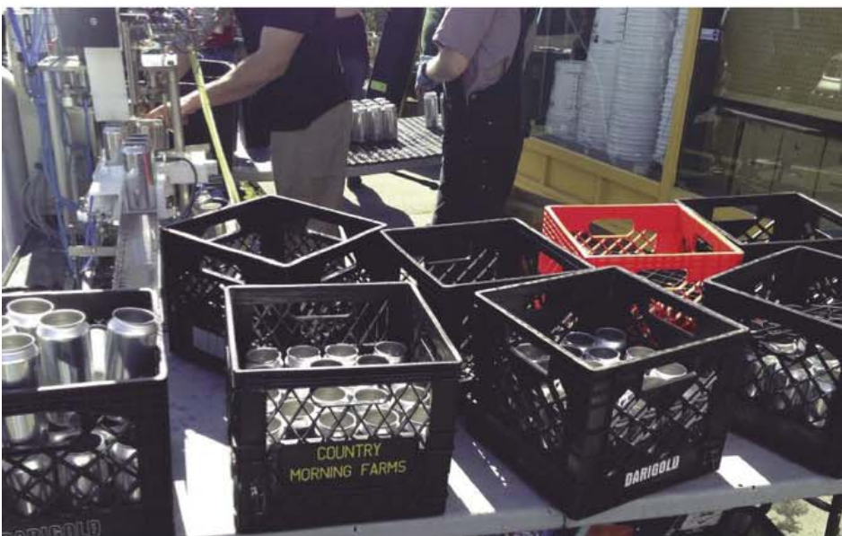
Mobile canning units most often work with 16-oz. unprinted aluminum cans, but may also use 12-oz. cans. The cost to can a 5-gallon (19-L) batch of homebrew is around $25 to $40.
