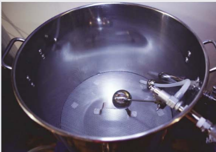
Following the mash, the sparge water moves from the HLT to the mash tun using the first pump, while wort is extracted from the mash tun into the brew kettle using the second pump. A Blichmann AutoSparge (center) helps ensure that the mash tun doesn't overflow.
