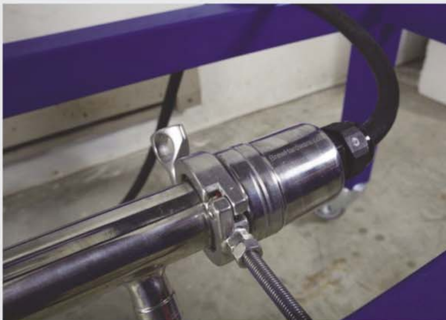
In addition to the two hot water heater elements, this system utilizes a stainless steel RIMS (recirculating infusion mash system) tube. The RIMS element has a tri-clover ferrule on each end for easy installation as well as disassembly for cleaning and sanitizing.
