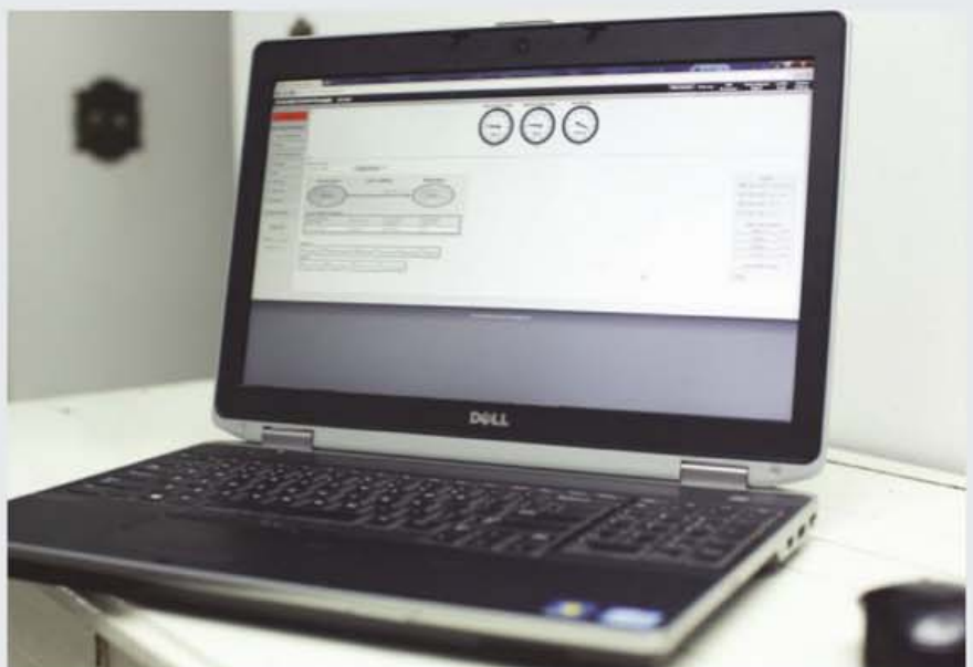
The BCS-460 unit that Trent chose for his system has a Web-based interface where he can glean lots of information at a glance. This includes current temperatures as well as running processes. You can also configure timers as well as buttons to completely stop all processes.
