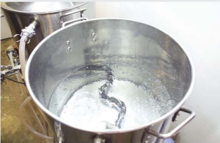
By installing and wiring the heating elements this way, the electric parts of the element are enclosed for safety and the kettle is grounded. This design also ensures that your vessels are sanitary as no trub or debris can gather, and the parts can be removed for cleaning.
