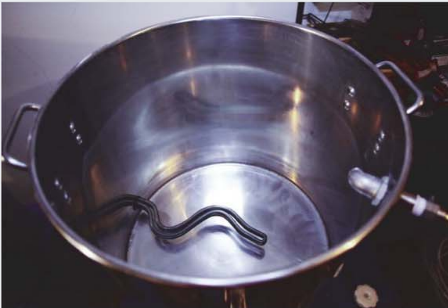
The heat used for boiling water and wort in Trent's all-electric system comes from inside the hot liquor tank (HLT, above) and the boil kettle in the form of two ultra low watt density (ULWD) water heater elements. The devices are installed using tri-clover fittings.
