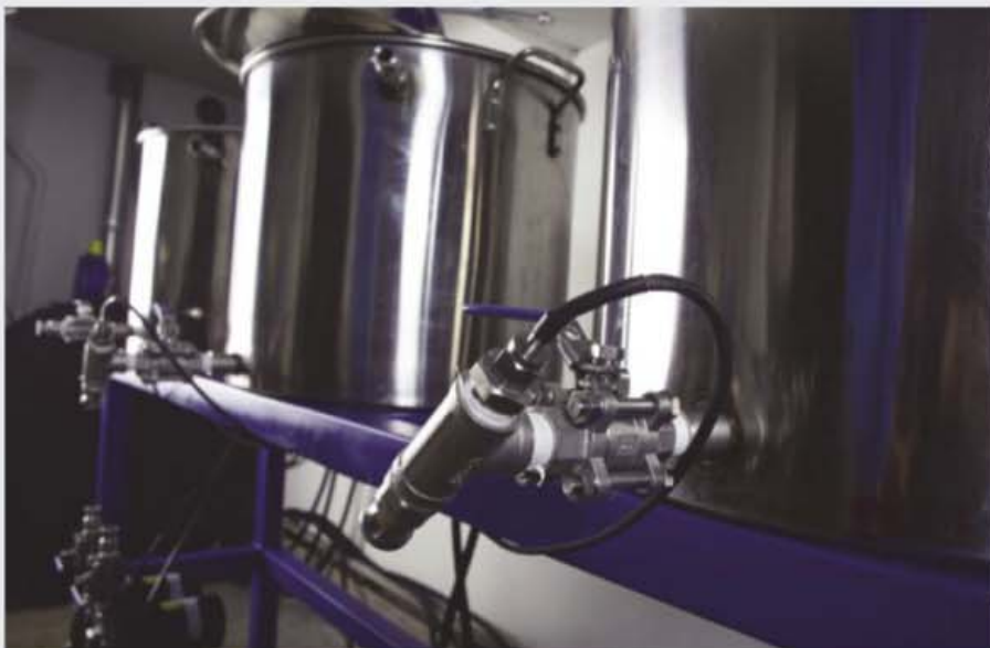
The temperatures in the boil kettle and mash tun are monitored and controlled by two temperature probes installed in the front of the vessels, which report back to the BCS-460. This allows Trent to precisely control his mash temperatures and increase them for mash out.
