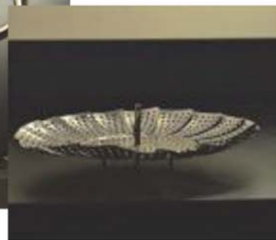
A simple vegetable steamer, commonly found in most kitchens, can become a false bottom when the middle post is removed.
