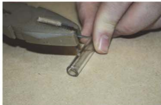
Poke small holes in your cut length of cane with a small, sharp object such as a finishing nail.
