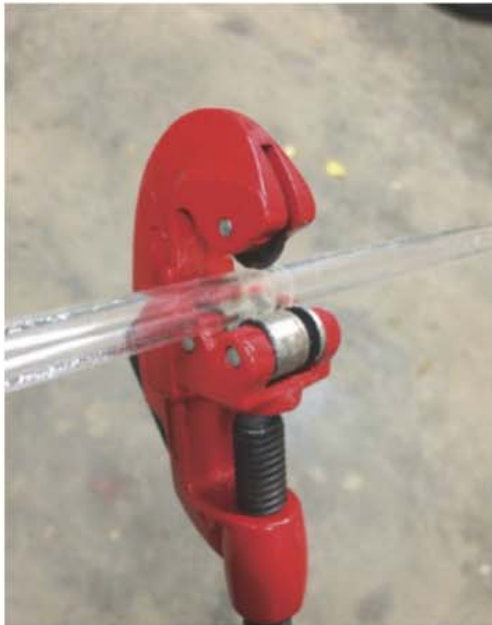
Cut the racking cane with a tube cutter or other sharp instrument. Use little to no pressure as the cane can crack.
