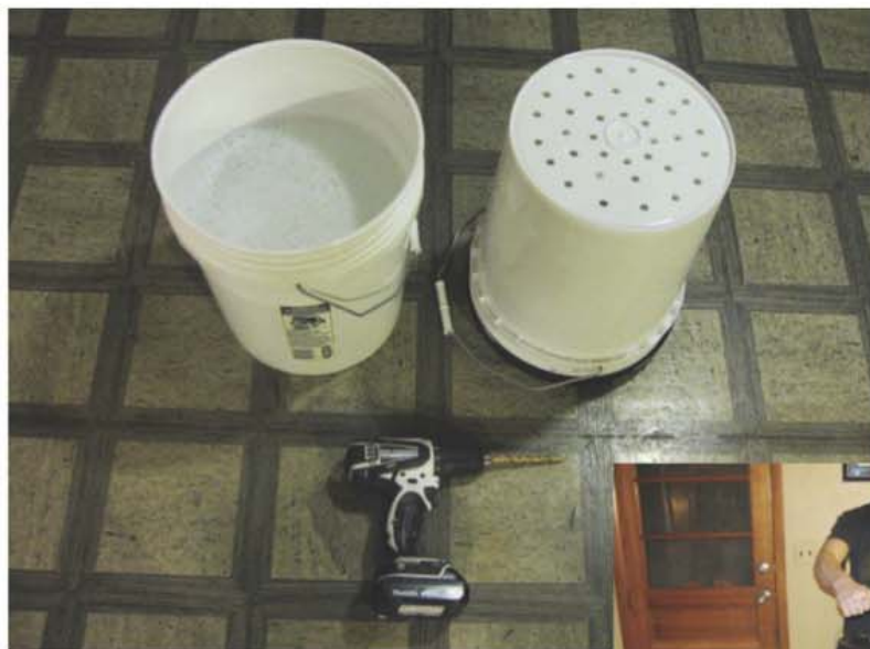
This easy sanitizing bucket setup requires only two 5-gallon (19-L) buckets and a hand drill.
