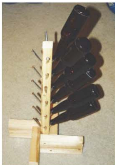
The "arms" of the tree are simply stainless steel nails covered with vinyl tubing.
