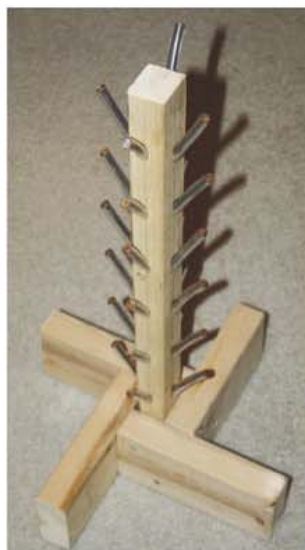
The base of the bottle tree is made with 2x2 and 2x4 lengths of lumber.
