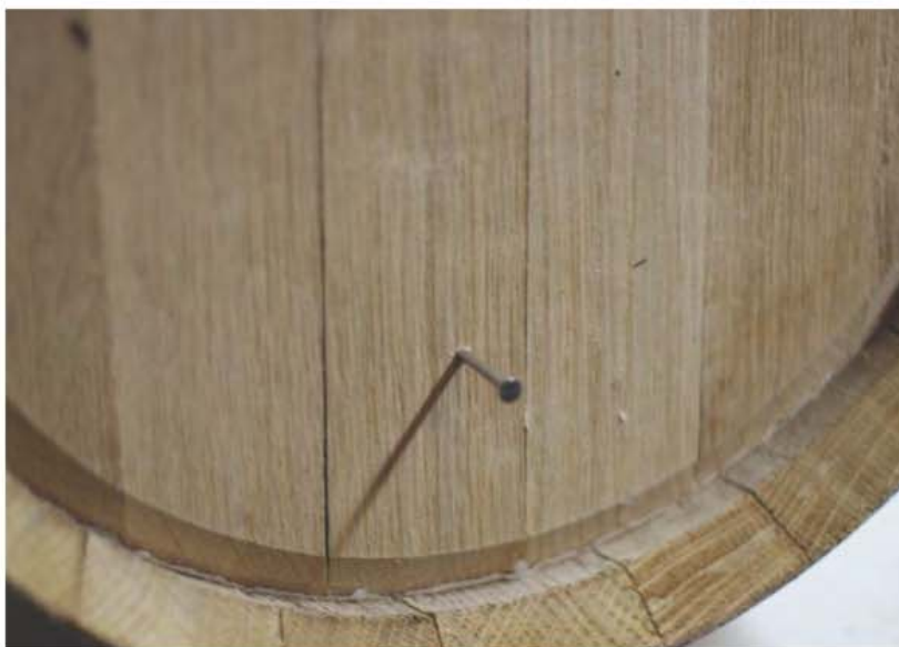
To prevent exposing your homebrew to air when sampling, drill a small hole and use a stainless steel nail to make a sampling port that you can easily open and close.
