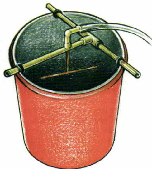
A sparge arm, resting above your mash-lautertun can deliver a steady rain of hot sparge water down on your grain bed.
