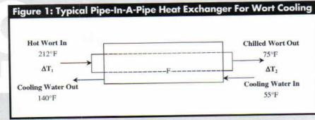
Let's work through an example to illustrate how these equations can be used to predict the amount of time it will take to chill your wort using a counter-current wort chiller.
