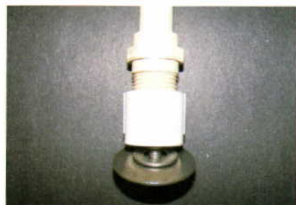
The large washer and small washer ride against the carriage bolt head.
