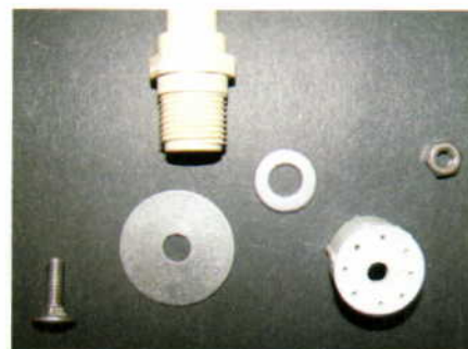
A carriage bolt (far left) holds the assembly together.
